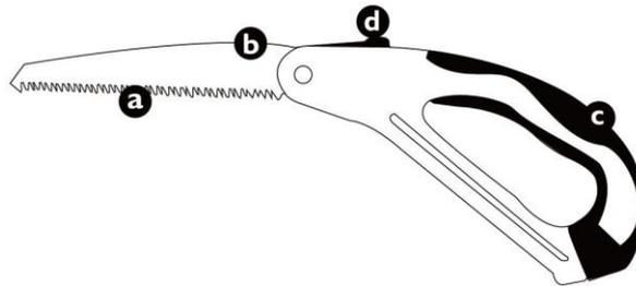
**a** Ultra-sharp triple-edged teeth can cut 5 times faster than the conventional saw blade.
