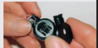
Position the casing lid and press down
