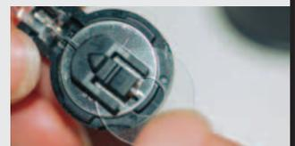
Plastic disc between switch and batteries
