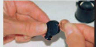
Open the casing with a small coin
