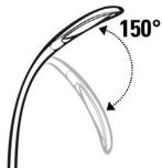
The neck of the lamp can be adjusted vertically (up/down) within a 150-degree angle.
