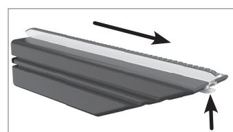
3. Place the grinding insert against the dry joint. Then slide it back and forth **WITH SLIGHT PRESSURE**. This loosens the dirt.
