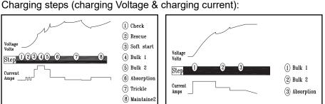
The battery charger must be connected to the battery according to the instructions above.
