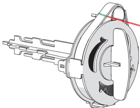
EN Cut the bandage carefully in the spring chamber
