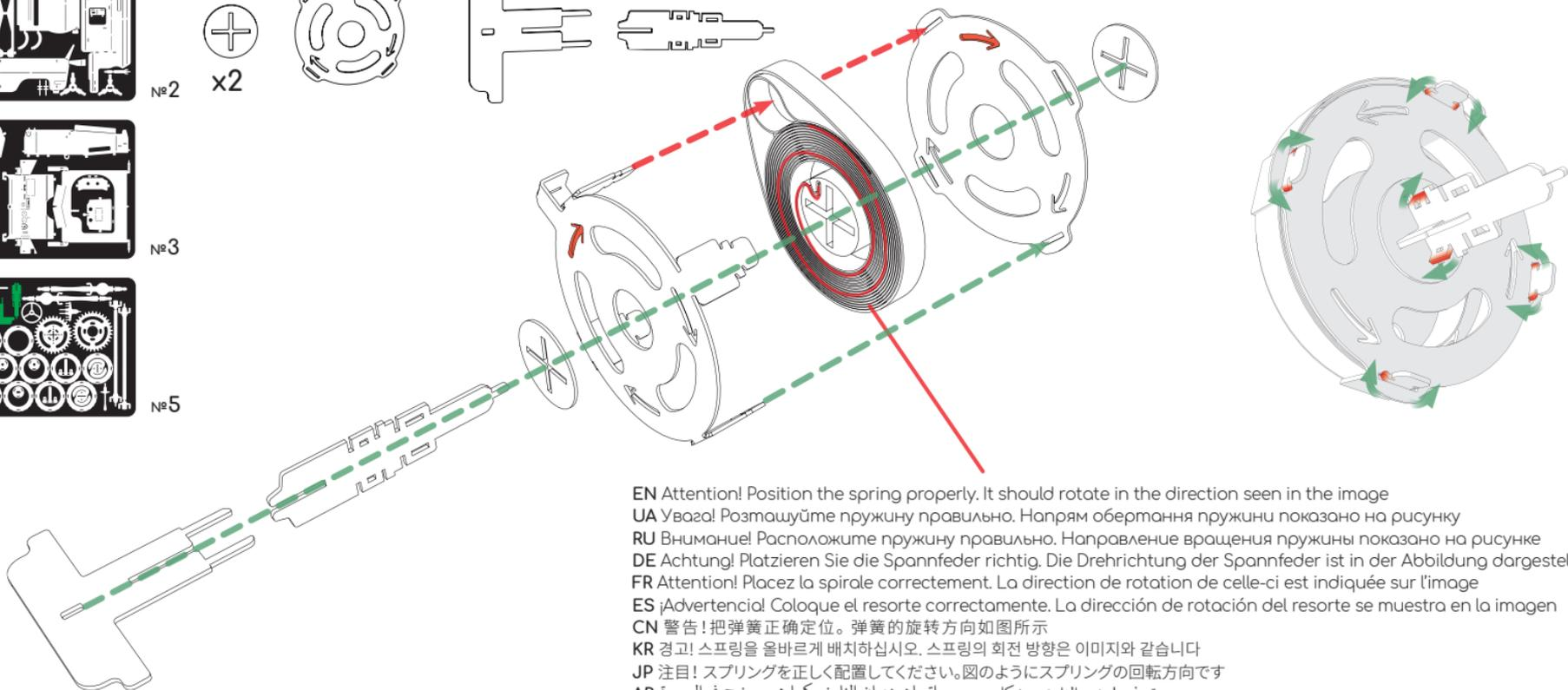
EN Attention! Position the spring properly. It should rotate in the direction seen in the image
