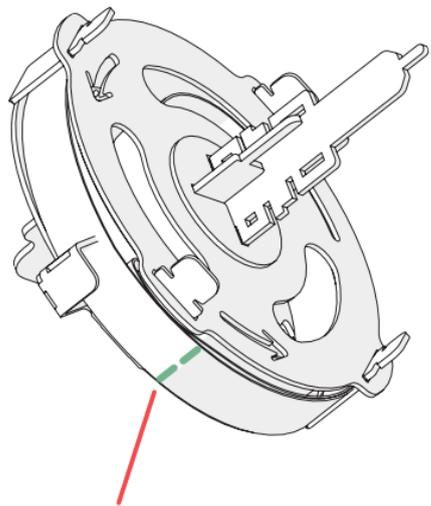
EN Remove the bandage from the spring chamber
