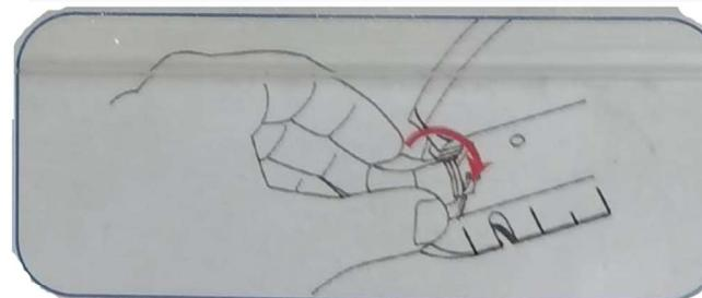
5. Place the tool flush against wall and use bubble level to adjust for straightness. Push down forcefully on grey button to dispense peg into wall.
