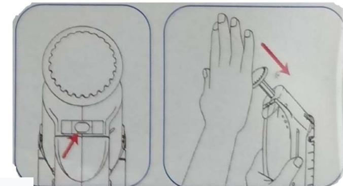
6. To remove a peg from the wall, line the removal notch up with the peg and pull away from the wall.
