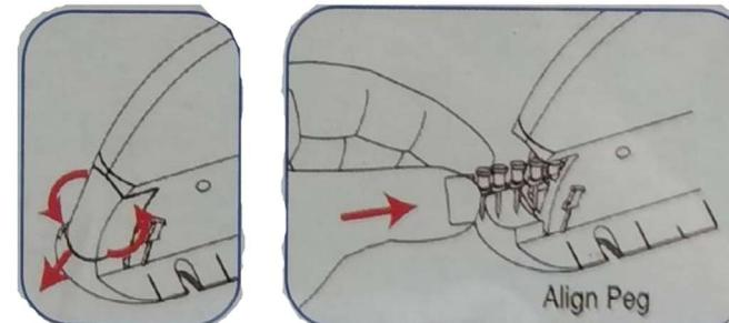
4. Replace end cap and turn it clockwise to lock into place.
