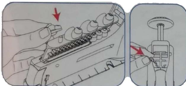
3. To load peg strip for use, turn spring loaded and cap counterclockwise to remove, and slide remaining peg strip into the compartment. Peg strip must be angled in the same direction as the peg icon at the end of the device.
