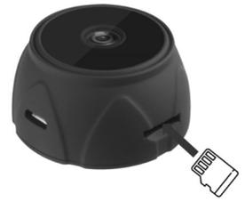
The TF card must be 8GB or above, and the format is FAT32. NTFS cannot be used normally. Data cannot be saved normally less than 8GB. If 64GB or 128GB card is used and the card is not FAT32 format, the device will automatically format the card when it is turned on. Please pay attention to data security.
