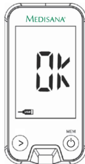
3. After successful transfer, "OK" appears in the display and the device emits an acoustic signal.
