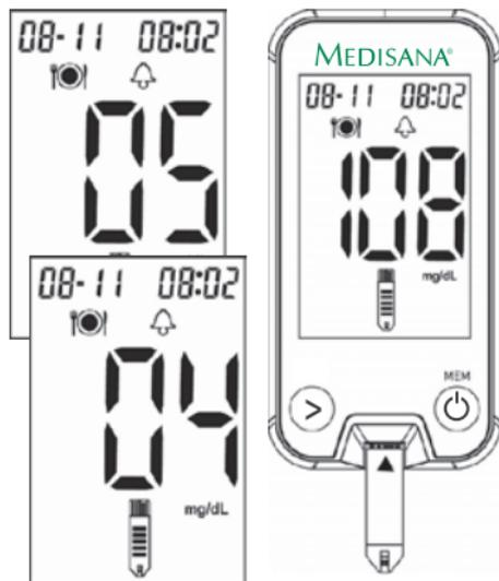
6. When a sufficient amount of blood has been absorbed by the reaction cell you will hear a beep and in the display "00" is shown.
