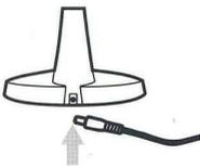
Connect the adaptor into the rear hole of the lamp base and insert the plug in a socket. **Note:** The adapter is exclusively used for this product. It cannot be used on other electric appliances.
