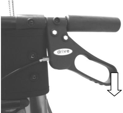
For parking the walking device press down the brakes until they click in the parking position (see picture). For unlocking the brakes pull them upwards towards the handgrips until they are unlocked (both brakes are in a middle position).
