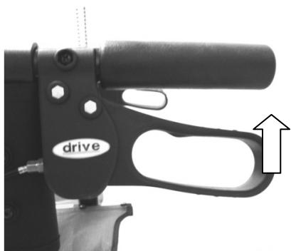
For braking the walking device pull both brakes upwards to the handgrip (see picture).
